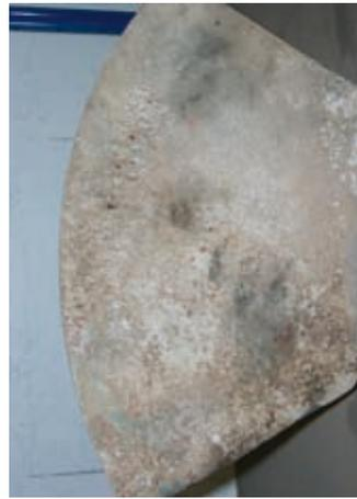
Photo 21. Kaplan turbine blade, manufactured without hydraulic laboratory techniques, eroded by cavitation after a few months operation
