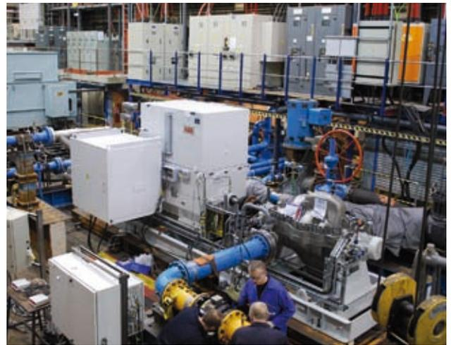
Photo 8. The Pelton turbine is set on the same shaft as a pump (the reverse osmosis process operates with a steady discharge)
