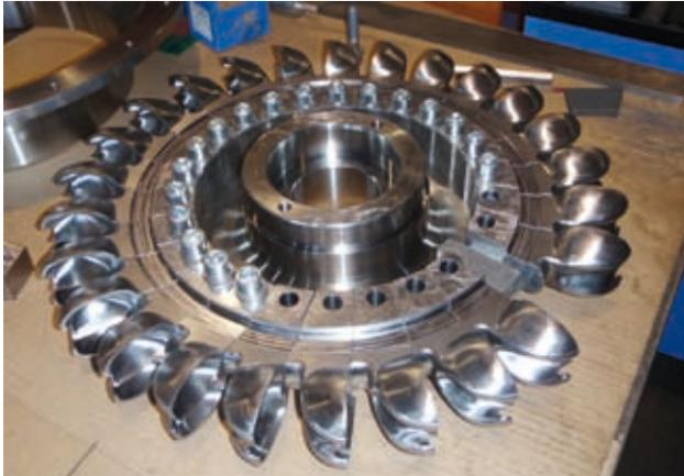
Photo 16. Achievement of a Pelton runner with mounted buckets (St Jean SHP plant, Switzerland, set in a drinking water network,  $\Delta Z = 373$  m,  $Q_n = 34$  l/s, 102 kW, 2009)
