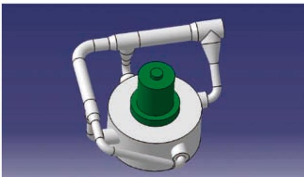
Figure 5. 4-nozzle Pelton turbine with a progressive flow acceleration to prevent waste from accumulating in the manifold
