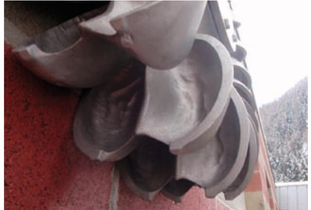
Photo 17. Pelton bucket worn out by sand particles (case study n°11, Profray)
