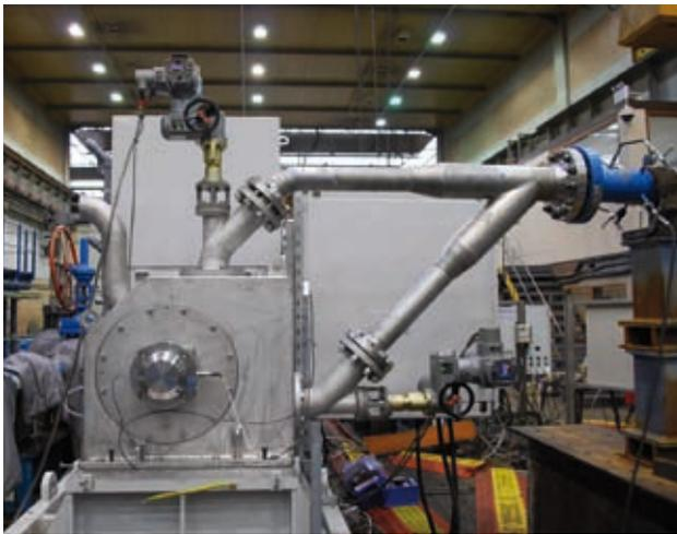
Photo 7. A 2-nozzle Pelton turbine developed for a desalination plant set in a test bench ( $\Delta Z = 735$  m,  $Q_n = 180$  l/s, 1.1 MW)
