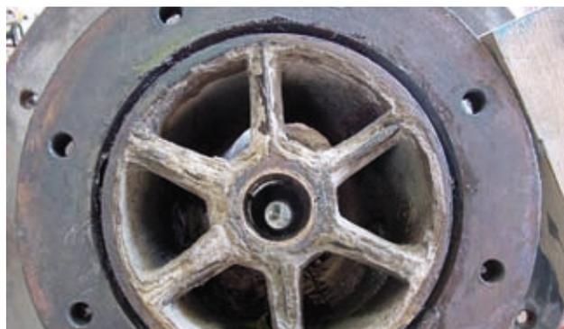
Photo 15. A nozzle guide vane, worn out by limestone
